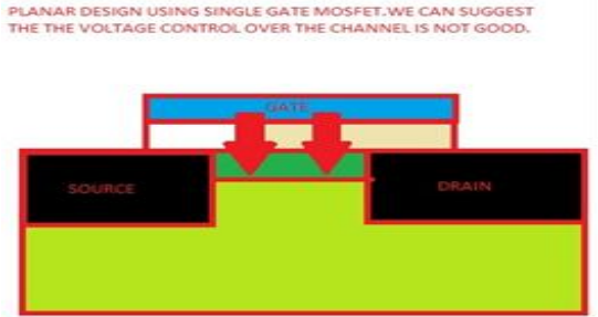
Figure 3. Poor Voltage Control in Planar MOSFET using Single Gate Control
