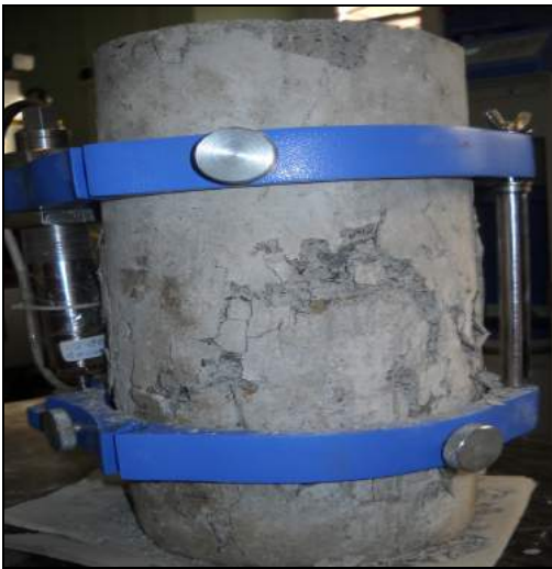
Fig. 3:- SFRC cylinder at failure
