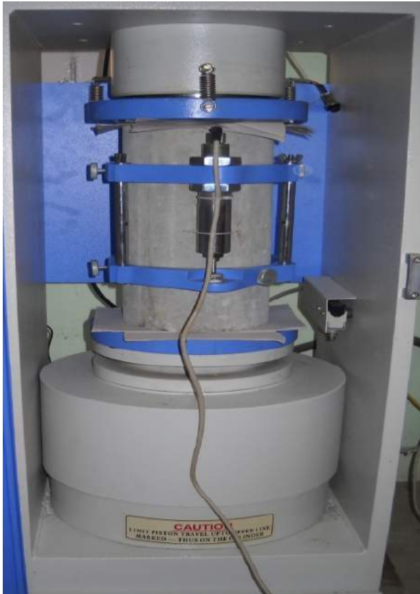
Fig. 2:- Specimen with Compressometer in ACTM
