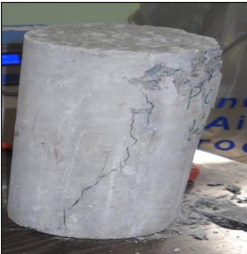
Fig.4:- Plain concrete cylinder at failure
