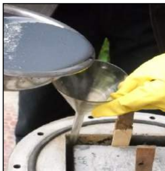
Fig. 2(c) – Sealing of sample using Epoxy sealant.
